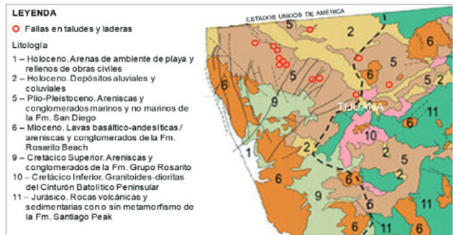
Figure 3. Slope and hillside failures recorded in the urban area of Tijuana (between 2010 and 2020).
