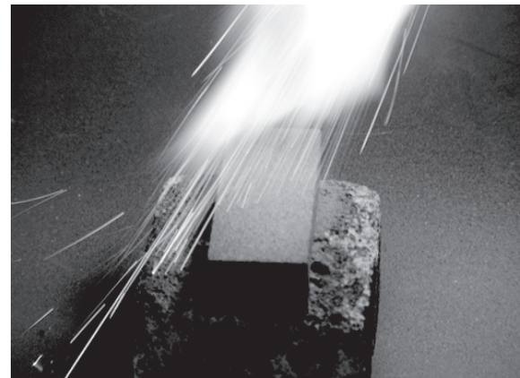
Figure 5. Deposits of alumina coatings through thermal flame spraying process
