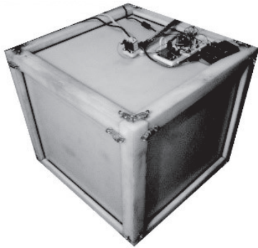
Figure 5. Cured Concretos Chamber
