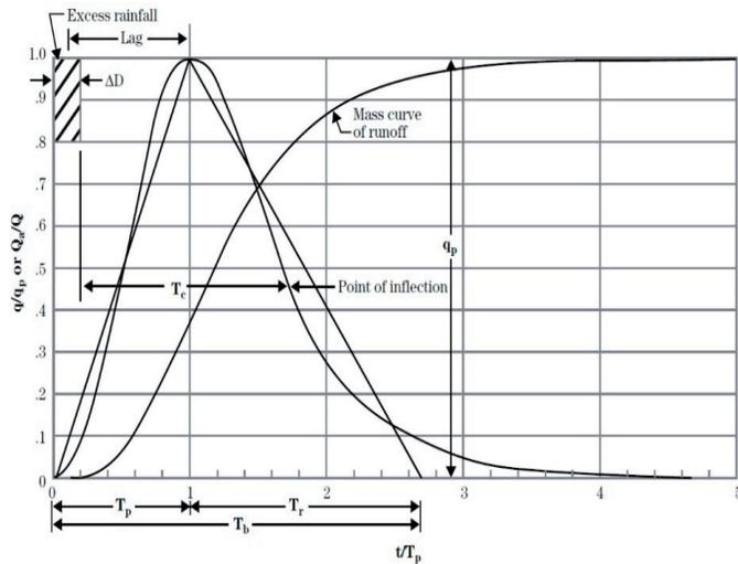
Figure 2. Dimensional unit hydrograph of the SCS
