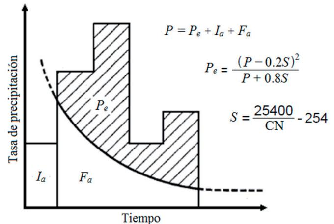
Figure 3. Variables in the method of precipitation abstractions of the SCS.
