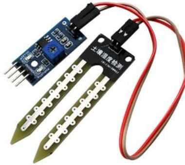
Figure 3. fc-28 soil moisture sensors
