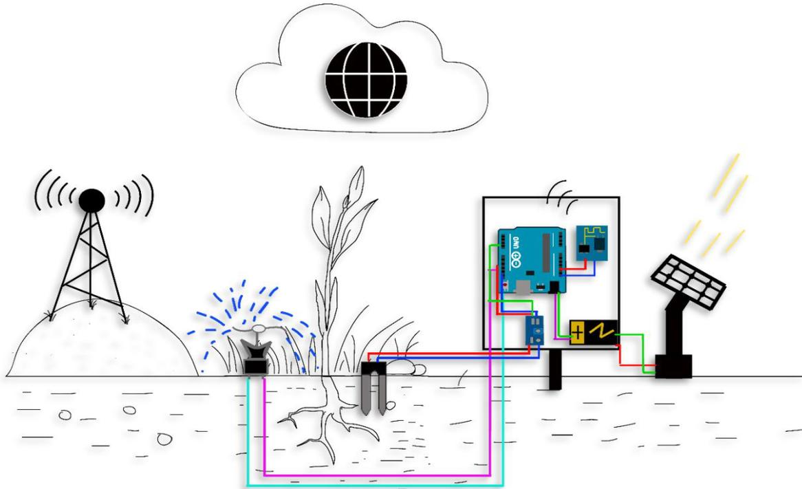
Figura 11. Schematic of project prototype model.
