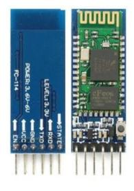
Figure 1. Bluetooth module HC-05 Source: [12].
