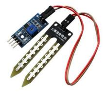
Figure 3. fc-28 soil moisture sensors Source: [13]
