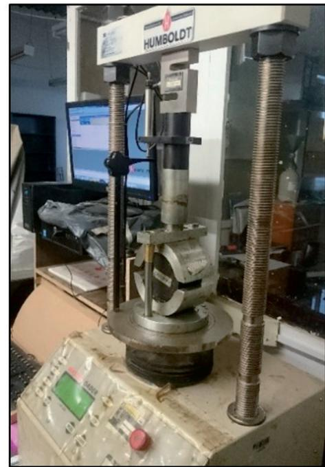
Figure 6. Equipment and test Stability and Marshall Flow
