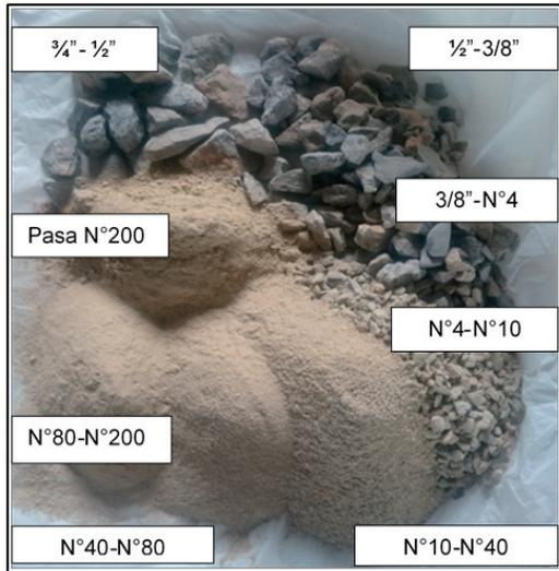
Figure 3. Aggregate dosage
