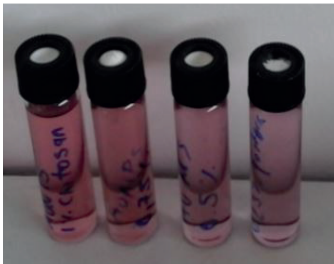
Figure 2. Synthesis of AuNPs at different concentrations of chitosan
