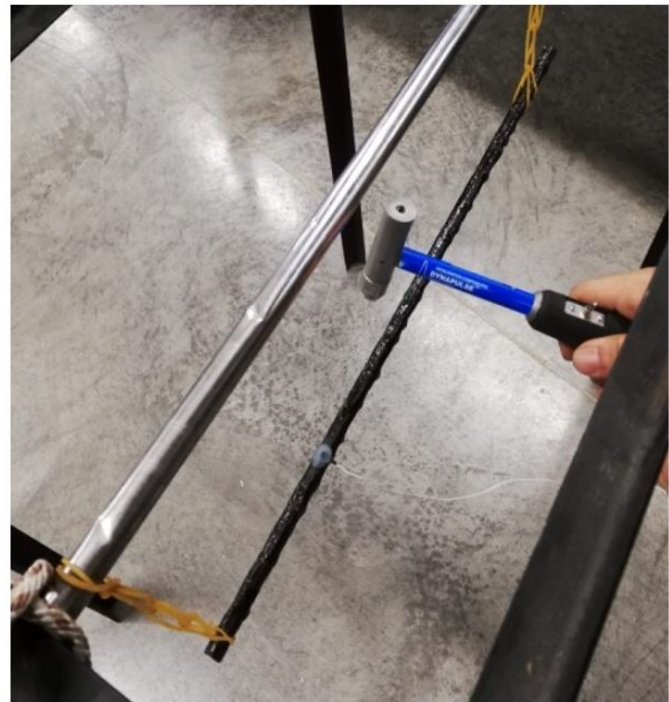
Figure 5. Experimental Modal Analysis (EMA), in free suspension condition for the axis of composite materials.
