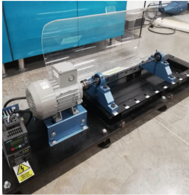
Figure 6. Carbon fiber shaft test bench. Source: Self-made
