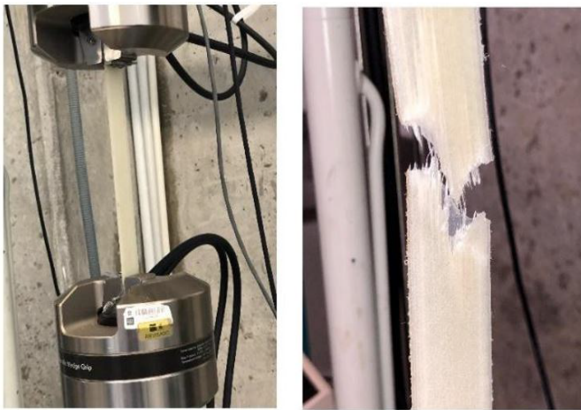
Figure 4. Tensile test and fracture
