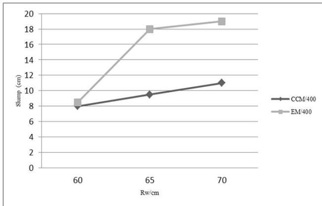
Figure 3. Slumps CCM-EM/400
