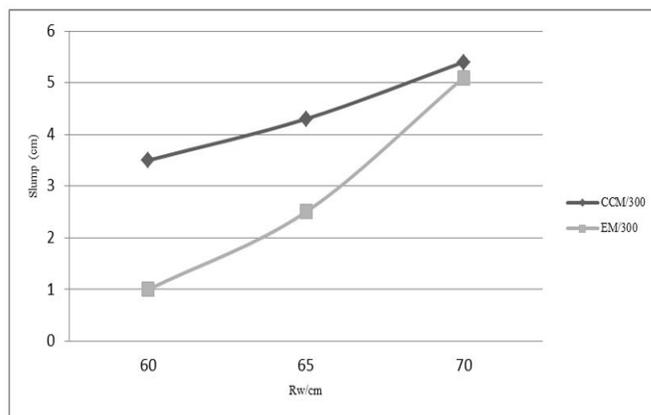
Figure 1. Slumps CCM-EM/300
