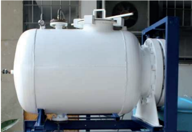
Figure 3. Pressure vessel modified in 2012 by [11], for wet welding simulation under water adapted for the extraction of samples for the measurement of the diffusible hydrogen content.
