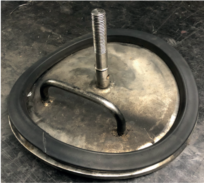
Figure 10. Manufactured inspection hatch
