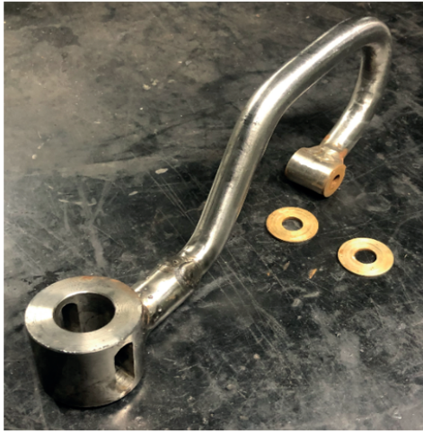
Figure 11. Articulated arm and manufactured washers
