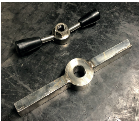
Figure 12. Rod and handwheel with welded nut
