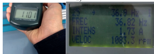
Figure 21. a) Speed change. b) Actual measured speed
