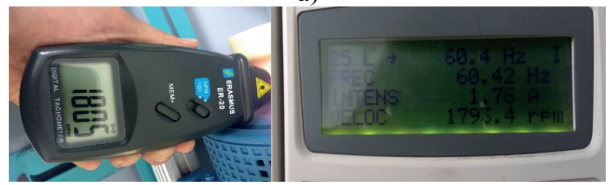
Figure 20. a) Speed change. b) Actual measured speed
