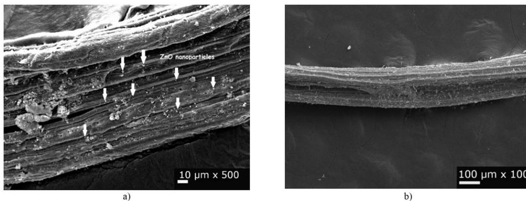
Figure 5. Scanning electron microscope of ZnO-Ex/fique fiber.
