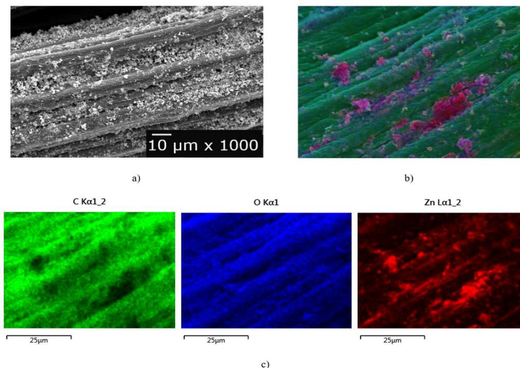
Figure 4. Scanning electron microscope, a) ZnO-In/fique, b) mapping images of ZnO-In/fique and c) EDS spectrum.
