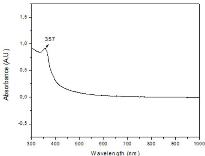
Figure 1. UV–Vis absorption spectrum of ZnO nanoparticles deposited in the fiber.
