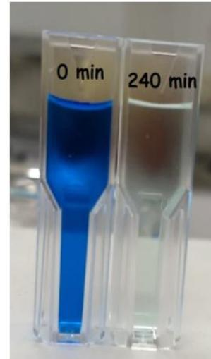
**Figure 8.** a) Color removal of IC solution at pH 2.5 catalyzed ZnO-Ex/fique fiber and ZnO-In/fique and b) Color removal of IC solution at pH 2.5 catalyzed by ZnO-Ex/fique for 0 min and 240 min.
