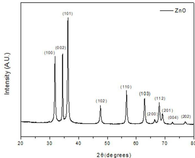
Figure 2. XRD spectra for the ZnO nanoparticles synthesized.
