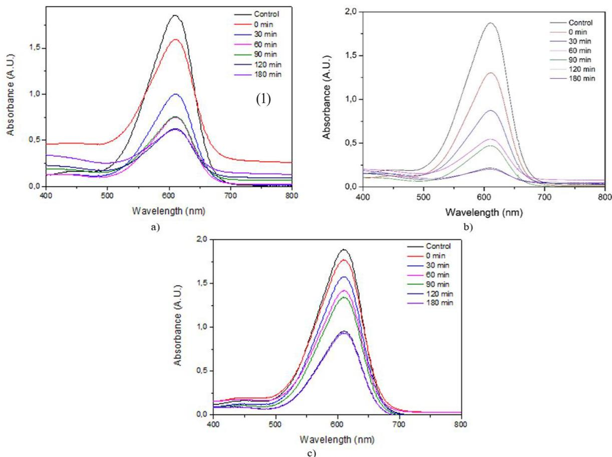
Figure 7. Absorbance spectra of color removal of IC dye with respect to time, a) ZnO-In/fique, b) ZnO-Ex/fique and c) ZnO nanoparticle.
