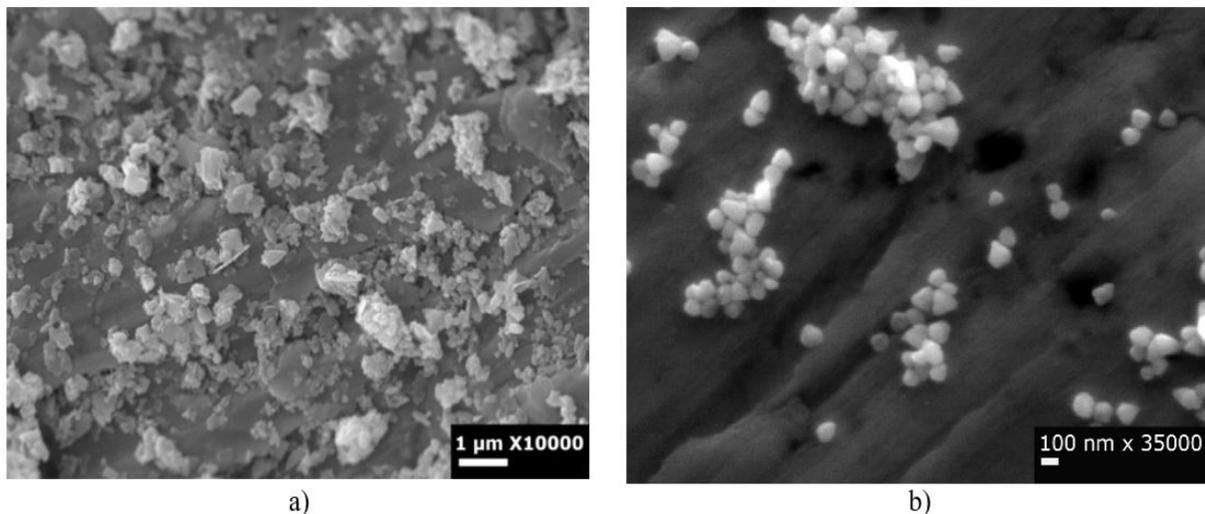
Figure 3. Scanning electron microscope of ZnO, a) Uncalcined nanoparticles (ZnO-In/fique) and b) Calcined nanoparticles (ZnO-Ex/fique).
