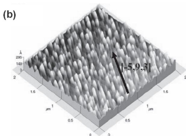
Figure 4. (a) Schematic figure of InAs-SAQDs structures grown on InGaAs stressor layers. (b) AFM image of the surface of a sample with 1.8 ML of InAs.
