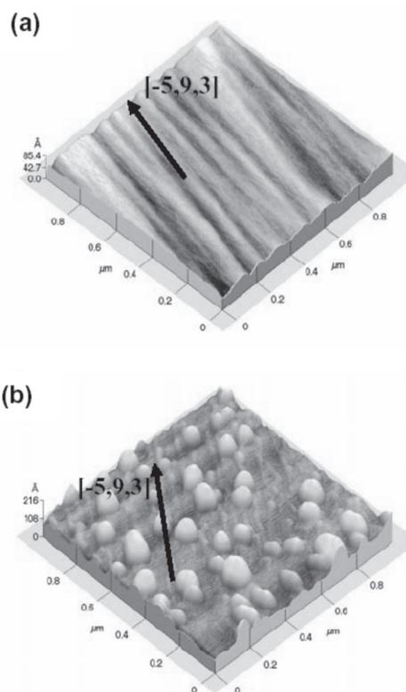
Figure 3. AFM images of the surface of samples with: (a) 1.8 ML of InAs, (b) 3 ML of InAs grown directly on
