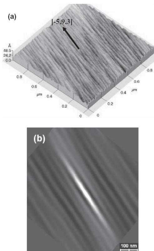
Figure 1. (a) AFM image of 80 nm-thick GaAs layer grown on GaAs(631)A substrate. (b) Autocorrelation function of the image in (a)
