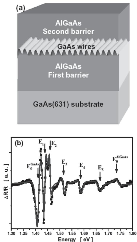
Figure 2. (a) Schematic figure of the quantum wire structure. (b) Photoreflectance spectrum from SAQWRs at 300 K.
